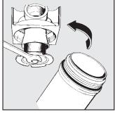
To clean or replace the filter element unscrew the screen of the centrifuge assembly. Use a no. 3 compass spanner to unscrew the bowl.
