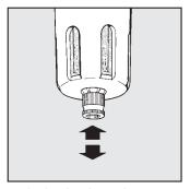
With the knob in the centre position, the drain is semiautomatic. The drain operates when the bowl is not pressurized and closes when it is.
