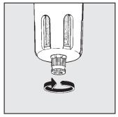
Turn the knob anticlockwise to close the valve with bowl pressurized or not pressurized.
